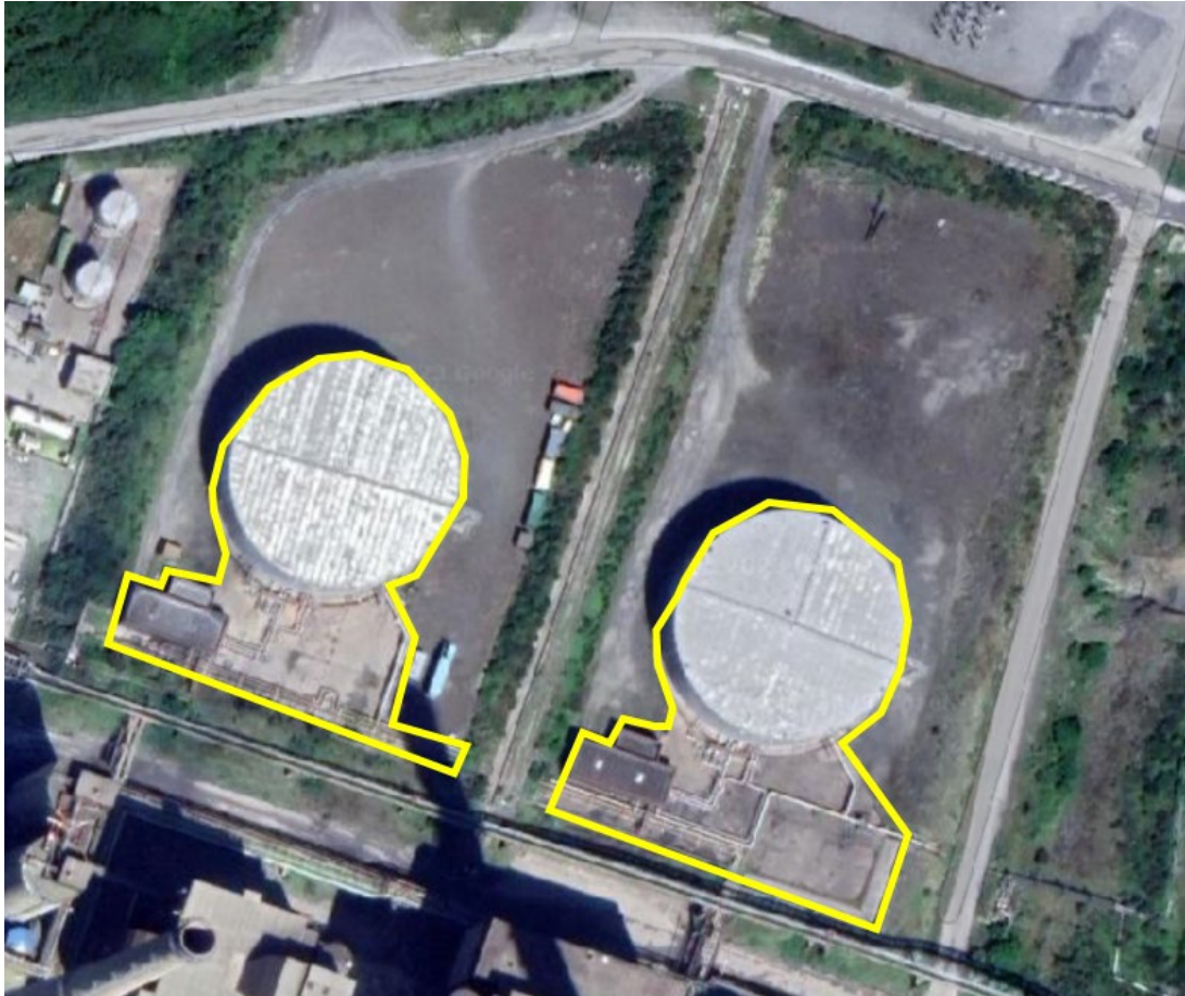
Figure 2.1 Aerial view of HFO Bunds with extent of impermeable areas in yellow outline
